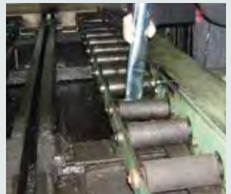
Vacuuming grinding sludge
